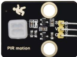
A black PCB module with a white PIR sensor component. It has a 3-pin header with pins labeled S, V, and G.                                                                          | Keyestudio PIR Motion Sensor           | 1 |
