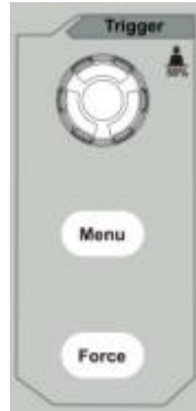
Figure 5-3: Trigger Control Area
